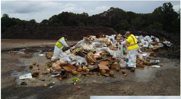
Contaminates are hand-picked out and remaining minor contaminates are grinded via the horizontal grinder and removed during the screening process.
