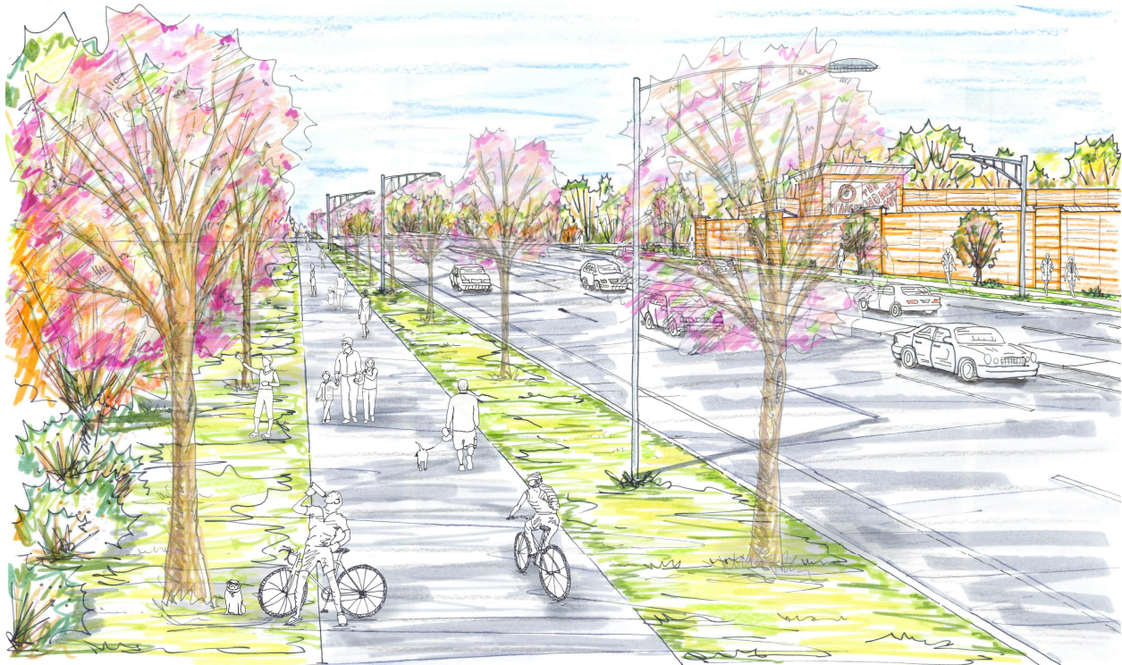
Figure 10 – Rendering of future shared use 10-foot path with 10-foot buffer
