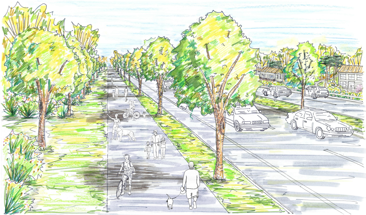
Figure 11 – Rendering of future 10-foot shared use path with 5-foot buffer
