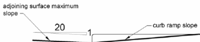
Figure 1-12: Counter Slopes at Ramp-Street Interface
