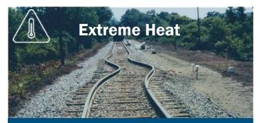
Extreme heat can reduce the number of active transportation users and temperatures above 85°F may cause rail lines to buckle and become misshapen.
