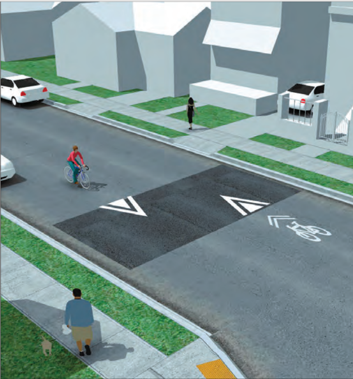
Speed humps use vertical deflection to slow motor vehicles and are among the most familiar traffic calming measures. | Source: NACTO
