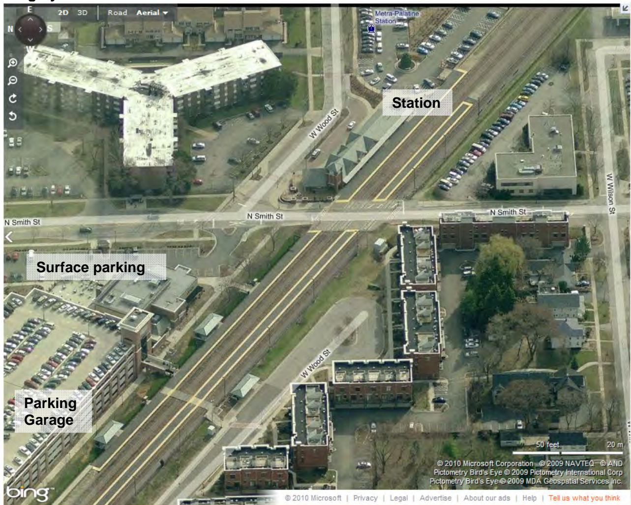
Palatine Station with two vehicular drop-offs, shared parking garage with “skyways” to platforms, pedestrian crossings to residential development
