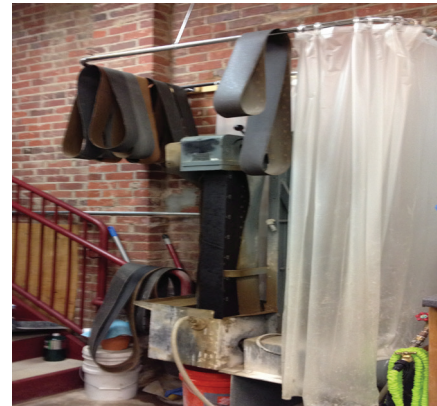
12) Cutting and polishing the rims with diamond saw and wet belt sander
