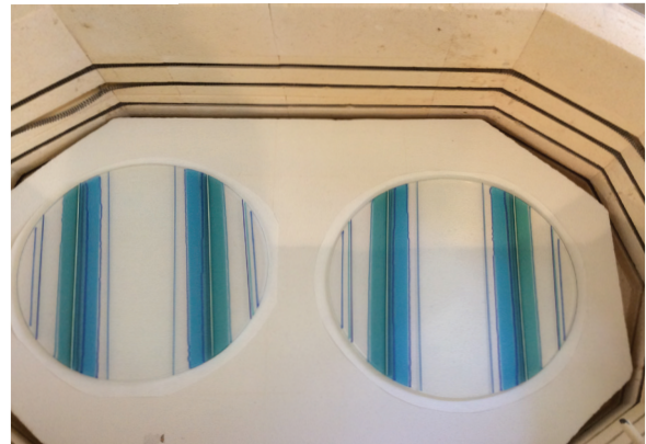
6) Ready for the first full fuse firing; 1475 degrees
