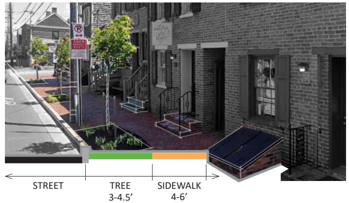
Sidewalk Condition 5: Curb + Street Tree + Sidewalk
