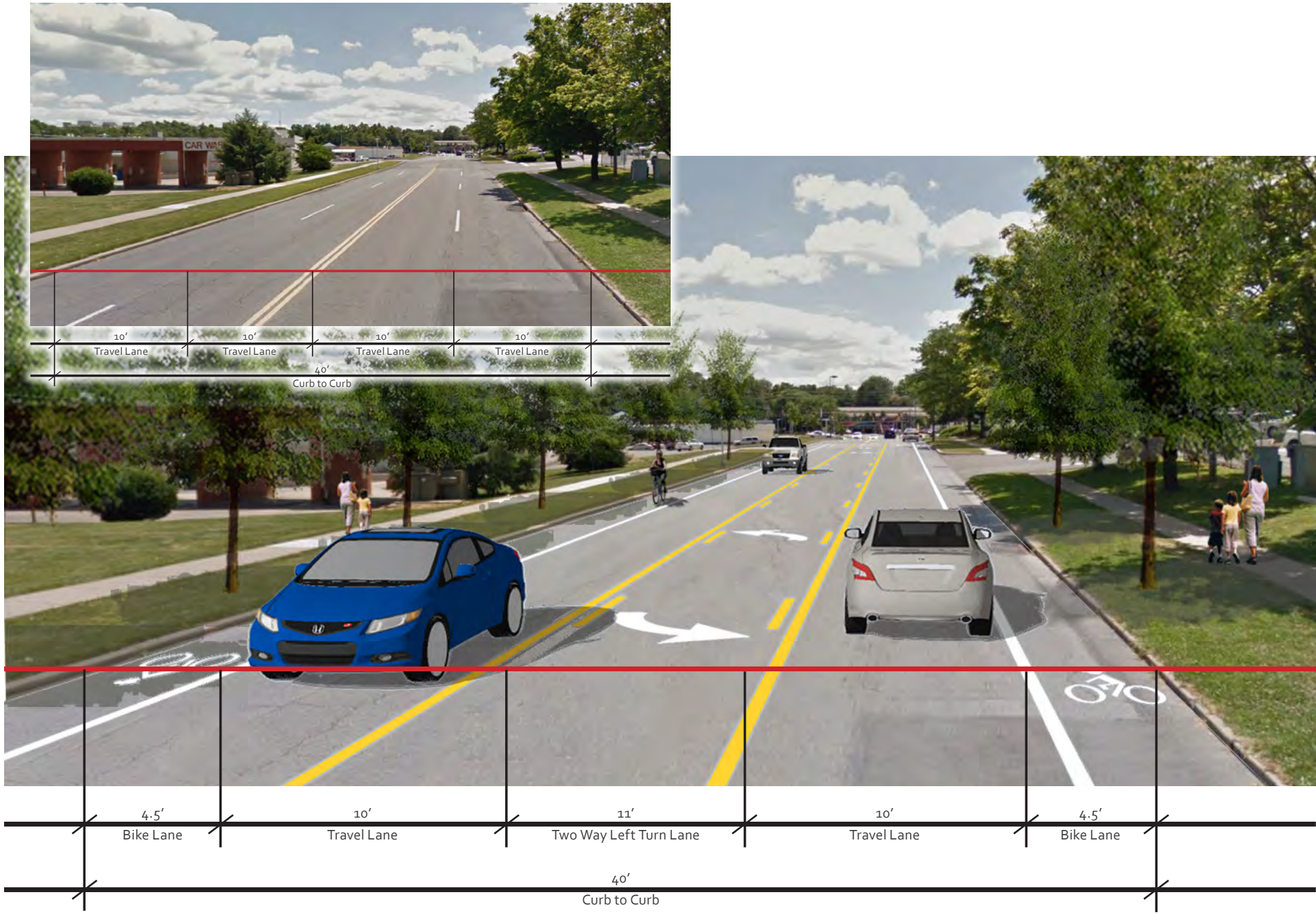
FIGURE 14 | WILLOWDALE DRIVE: RESTRIPIING AND STREETSCAPING OPPORTUNITIES (SIMILAR OPPORTUNITIES EXIST ON WAVERLY DRIVE AND MCCAIN DRIVE)
