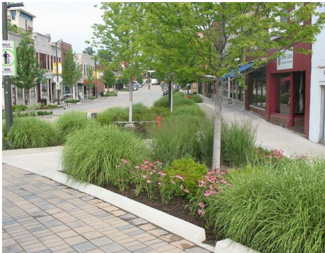
Lush streetscape planting with integrated stormwater management
