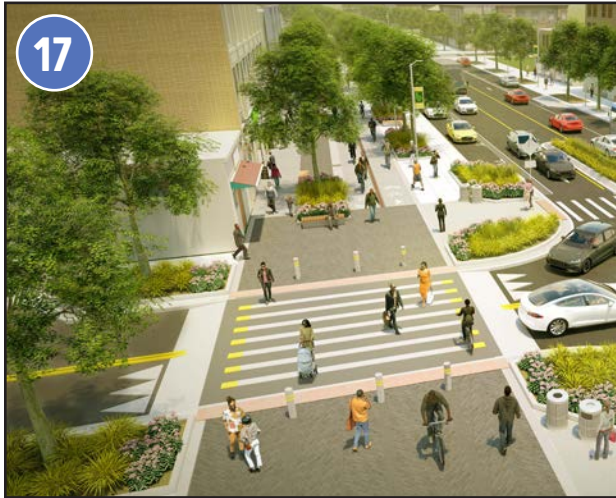
Examples of traffic calming at an intersection
