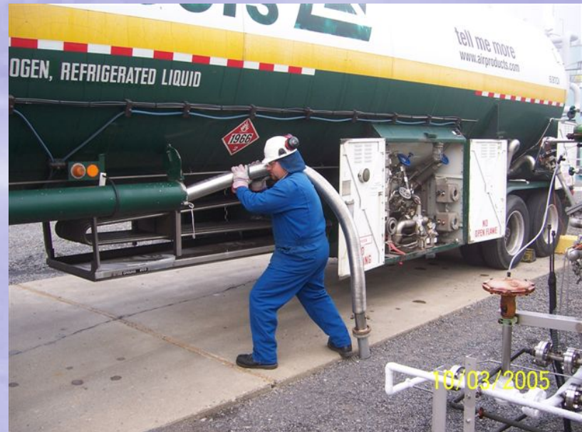
A delivery driver prepares to drop off a load of liquid hydrogen.
