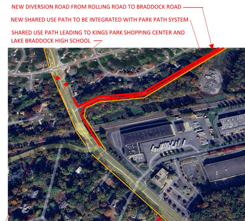
PROPOSED NEW TRAFFIC DIVERSION DIAGRAM INTERSECTION AT ROLLING ROAD
