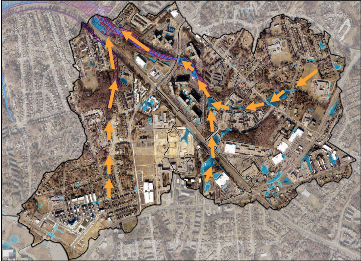
Figure 27: Primary flood and drainage corridor within a representative Focus Area. Orange arrows indicate the surface and stormwater flow direction. Adjacent green spaces, ponds, and public rights-of-way are prime search zones for volume-based BGI practices.
