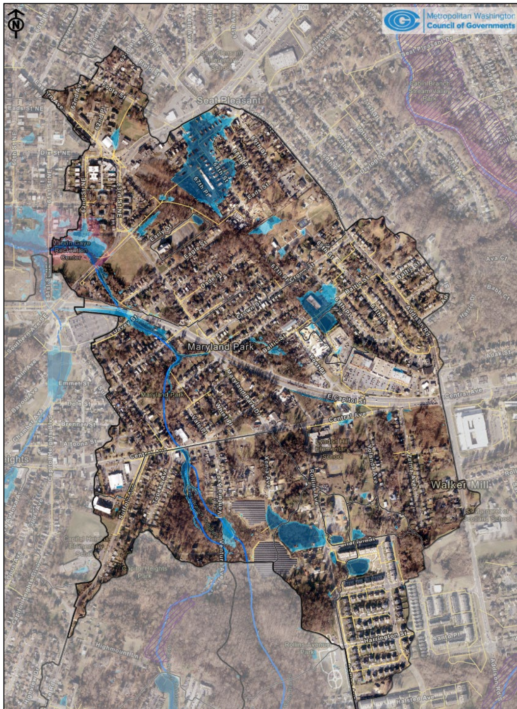
Figure 26: Example flood risk mapping within a Focus Area. Layers shown include storm drain infrastructure, Blue Spot analysis, and aerial imagery. In the District, similar maps used IFM outputs in place of Blue Spot data to better capture interior flood risk. Darker shades of blue represent potentially higher depth of inundation.
