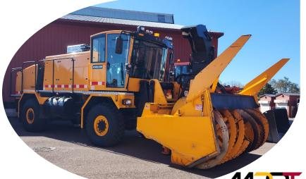
3,500 tons of snow removal capacity per hour
