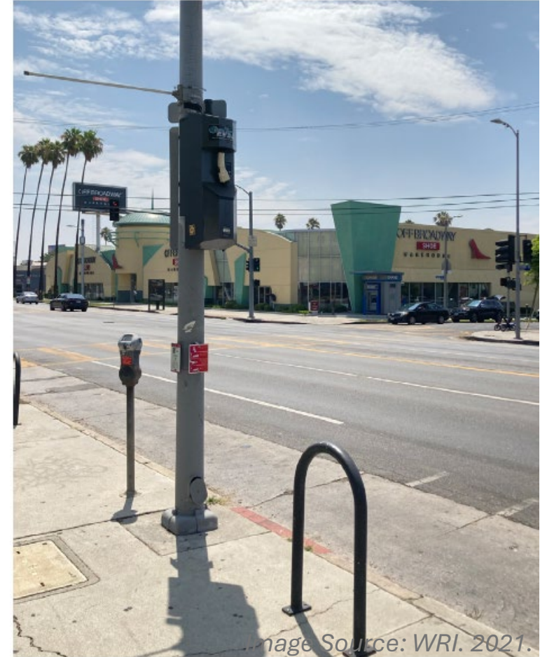
Elevated pole-mounted charger on streetlight pole in Los Angeles, CA
